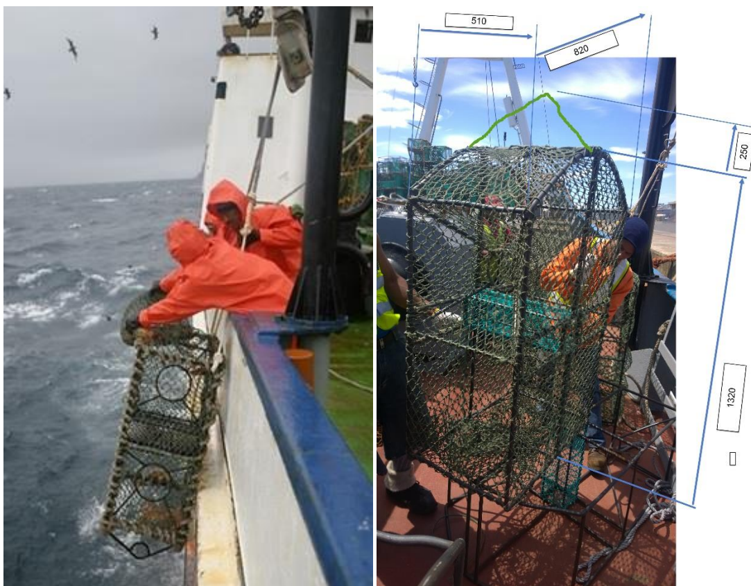
Figure 3. Monster trap retrieval and dimensions. Source: Ovenstone.
