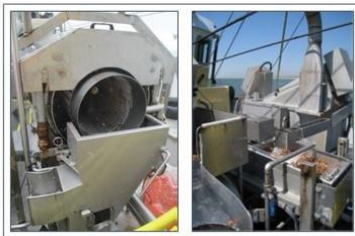
Figure 3.6-18 Sieving devices on board of shrimp vessels: coaxial sieving drums (left), trembling/shaker sieve (right) (Source: Steenbergen et al , 2015).
