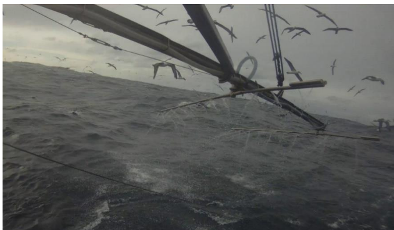
Figure 9. Seabird sprayers in situ (Source: https://www.afma.gov.au/environment-and-research/reducing-bycatch/bycatch-reduction-devices/seabird-sprayer )
