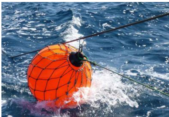
Figure 10. Warp deflector in situ (Source: https://www.afma.gov.au/environment-and-research/reducing-bycatch/bycatch-reduction-devices/warp-deflectors )
