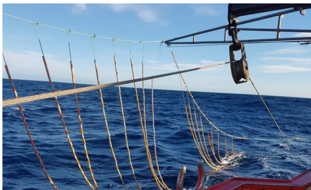
Figure 8. Bird baffle in situ (Source: https://www.afma.gov.au/environment-and-research/reducing-bycatch/bycatch-reduction-devices/bird-baffle )
