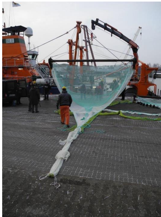
Figure 3 Example of a sieve net employed by a German shrimp vessel
