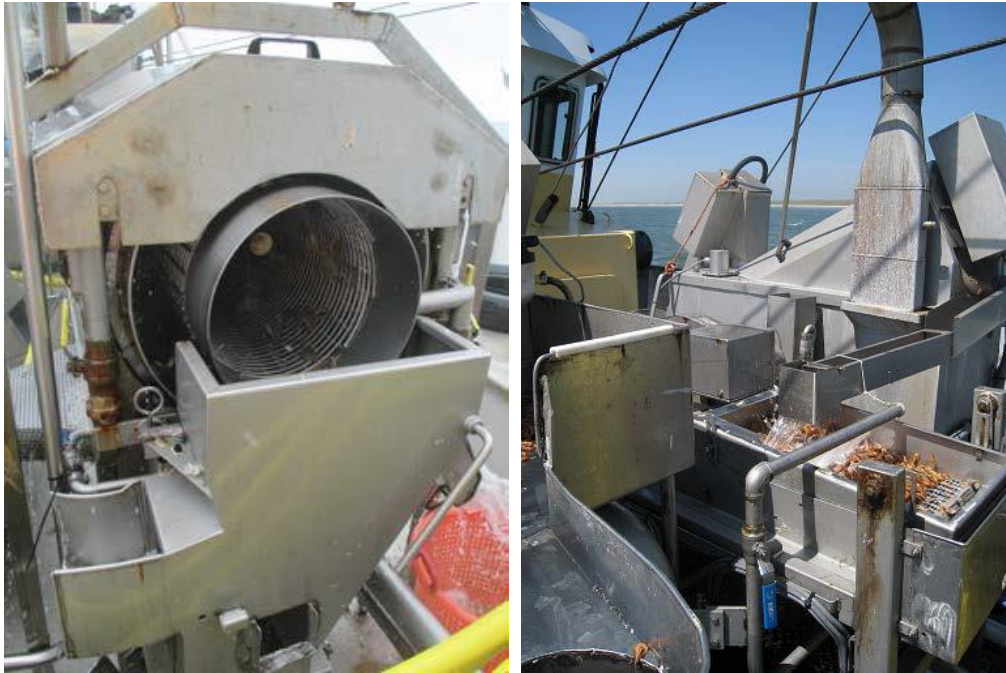
Figure 41 Sieving devices on board of shrimp vessels: coaxial sieving drums (left), trembling sieve (right) (Source: Steenbergen et al, 2015).
