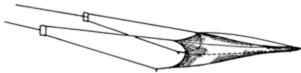
Figure 3. Midwater otter trawl (source: FAO.org)
