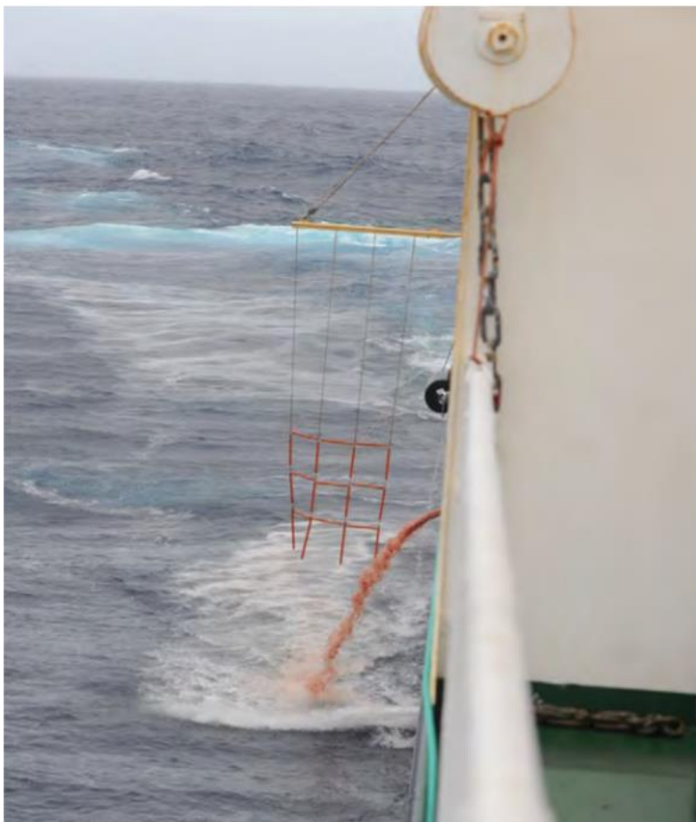
Figure 18. Bird bafflers that are supposed to keep the birds away from the trawl (Figure 5 in Raczyński, et al., 2016).
