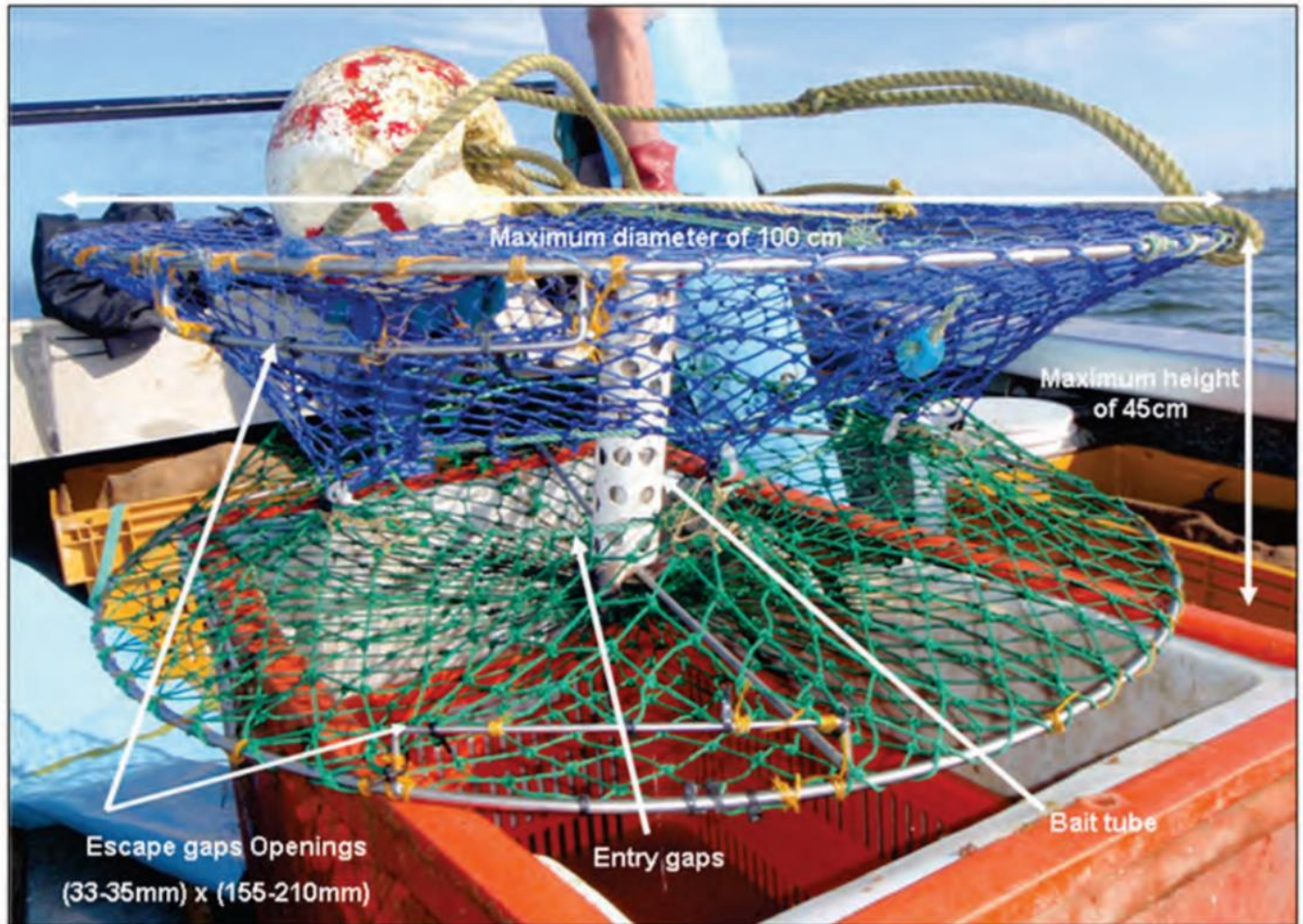
Figure 2: Commercial blue swimmer crab trap. From Johnston et. al. 2015
