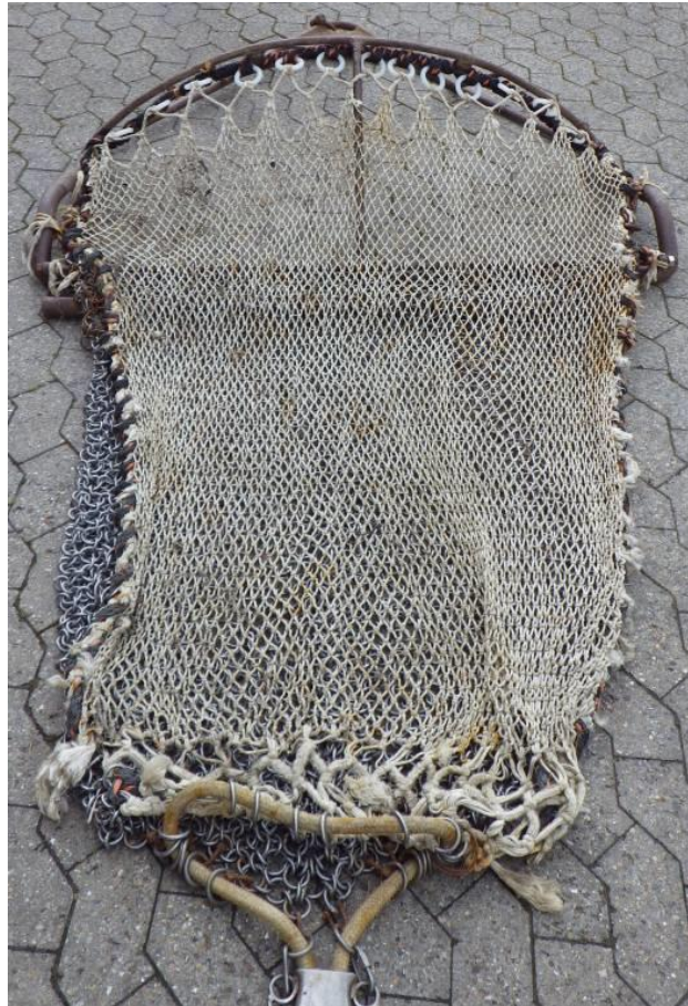
Figure 5: Picture of a standardised dredge gear used in DTU-Aqua research surveys showing top mesh panel (25 mm).
