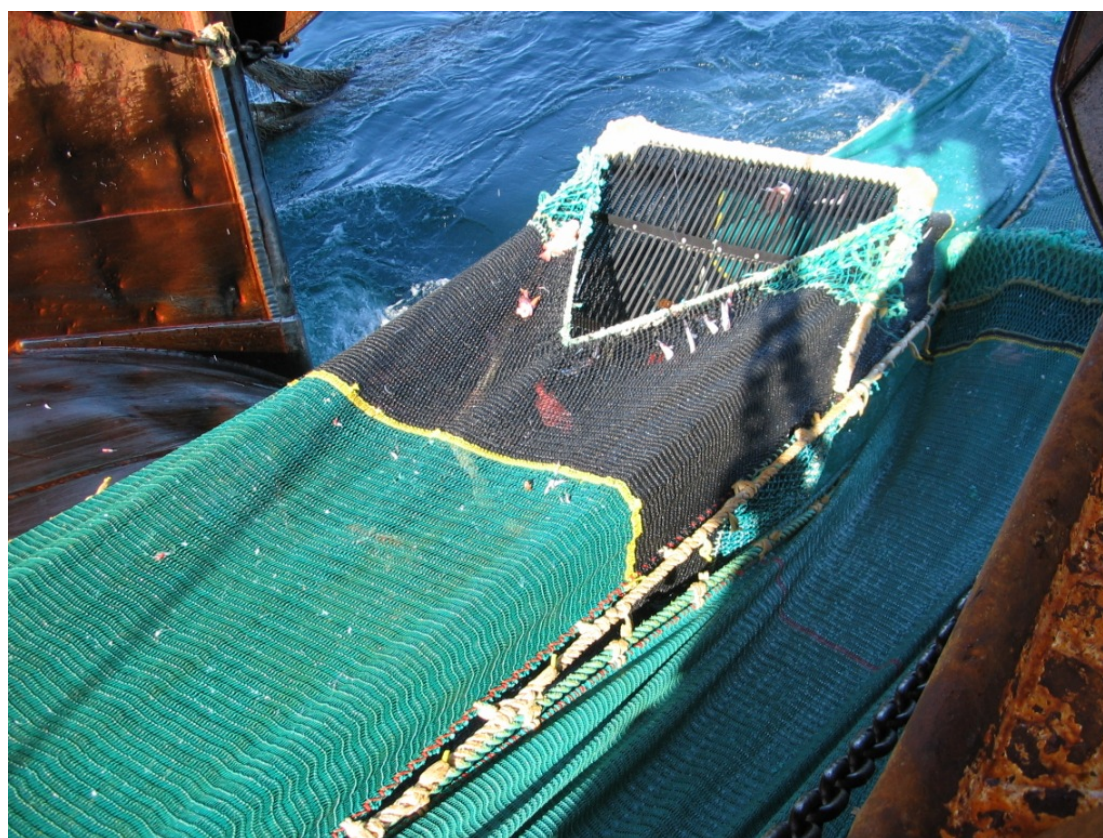
Figure 4: Sorting grid used on shrimp trawlers in the Barents Sea.
