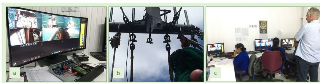
Figure 3.2.4: Images showing the on-board cameras and the CCTV review system: a) the hard drive coupled up, showing the six views from a single vessel; b) the camera installed on the trawl gantry; c) a member of the assessment team hearing how the CCTV footage is reviewed (images by T. Southall)
