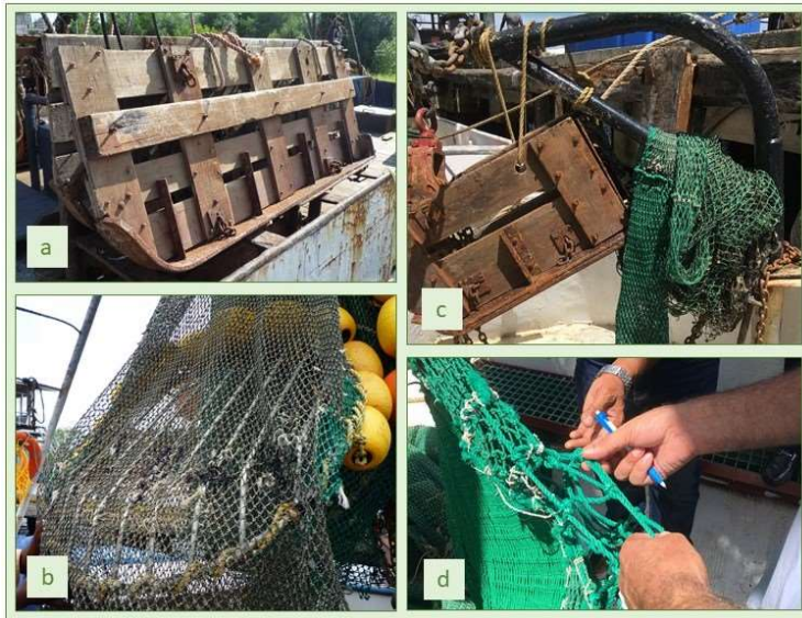
Figure 3.2.3: a) A typical trawl door; b) the TED; c) the small try-net; d) assessors examine the BRD (images by T. Southall).
