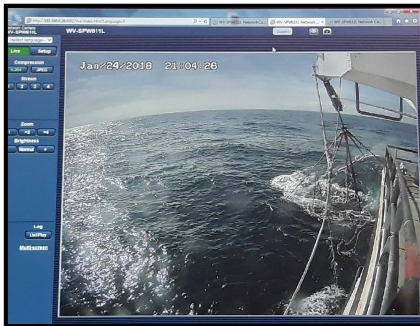
Figure 6: Screenshot of the camera system installed in the stern of the Saga Sea vessel to monitor the third wire for bird interactions. Source: Saga Sea CCAMLR observer report for the 10/11/17 - 28/03/2018 trip.
